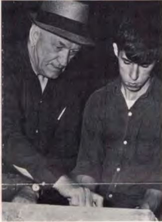
Jim Gray, Shop Instructor, for Barre's Apprentice School, helps an apprentice lay out a slant marker. Granite is contributed by the member-companies of the Barre Granite Association.
