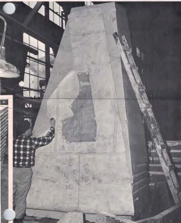
The huge Barre granite block stands on its base. Approximately 10 tons of excess granite have been removed by the giant Wells-Lamson Saw. Ferdinand Weber, the sculptor, is making preparations to remove additional excess granite by channeling. Weber is one of nearly 40 sculptors employed in the Greater Barre Area. He will perform most of his work on the statue within the Vermont Pavilion Expo '67 in Montreal where four million visitors will view his efforts.
