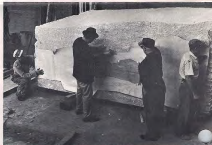
Ferdinand Weber, second from left, is shown laying out a large paper pattern on the block of Barre granite recently lifted from one of the Rock of Ages quarries. By outlining the pattern Weber provides guidelines for the Wells-Lamson Saw Plant personnel in setting up the huge block under the wire saw.
