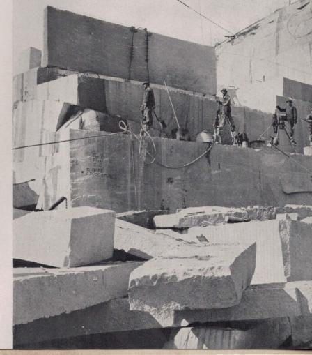
A perfect block of Select Barre Granite 40 feet long being drilled to make two mausoleum roof stones each weighing nearly 50 tons.
