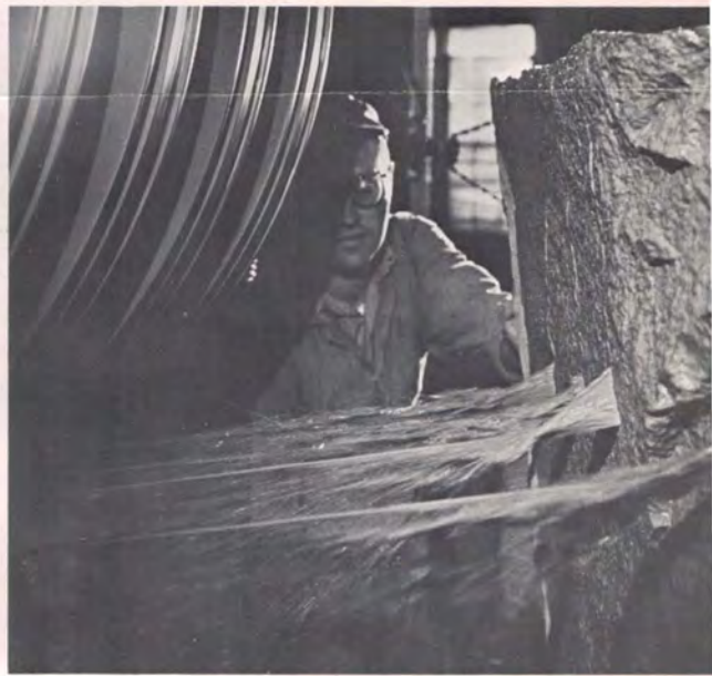
3. A block of Barre granite being wire sawed into slabs.
