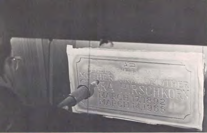
7. Sandblasting names and dates on a Barre granite memorial.
