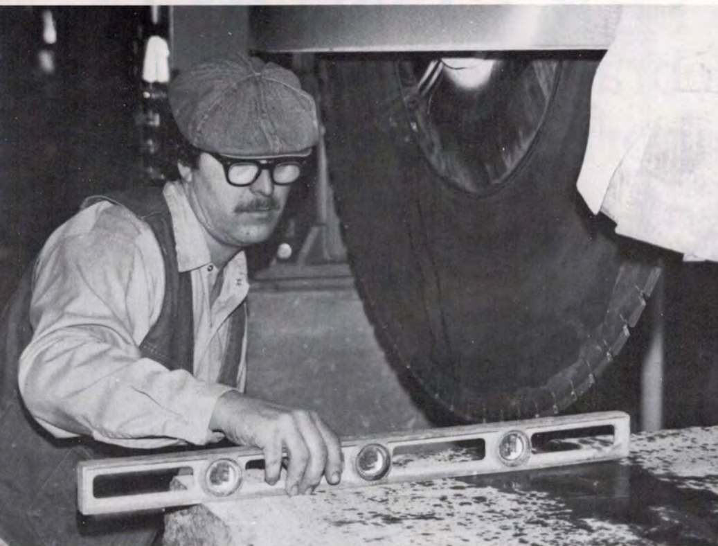
ROBERT RIVARD , President of Rivard Granite Company, lines up a slab of Barre granite on the company's new Ordway diamond saw. One of the smaller member-firms of the Barre Granite Association, Rivard Granite Company has been a consistent leader in designing more efficient methods of producing beautiful granite memorials.
